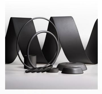
Crossflon® XF232 is black in colour and provides a good balance of properties for bearing applications. It has an extremely low coefficient of friction, a high level of chemical inertness and good wear resistance especially against soft mating surfaces. This material has higher creep resistance and thermal conductivity than unfilled PTFE to allow for greater loading ability and cooler running when used in dry conditions.
