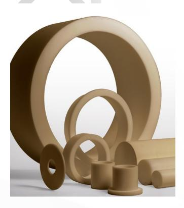
Crossflon® XF224 is gold in colour and has been specifically formulated to operate against soft mating surfaces such as aluminium, brass, mild steel, other plastics and stainless steel. This material possesses no hard or abrasive fillers, has a low coefficient of friction, good creep resistance and compressive strength along with very low wear rates in comparison to unfilled PTFE.
