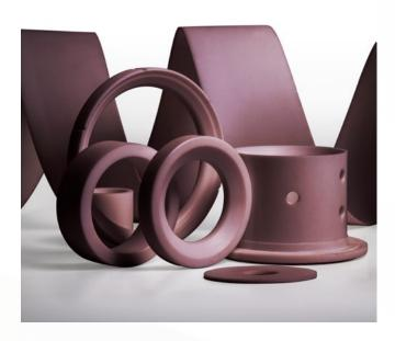
Crossflon® XF222 is primarily used in the manufacture of seals. It has excellent load and wear characteristics and is compatible with soft mating surfaces. This material is light maroon in colour and specifically formulated for use in food and drug contact applications with all components being FDA compliant.
